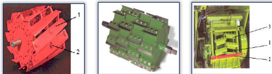
Figure 3 – Types of cutting drums. a) Chopping drum with spiral blades (New Holland 770); 1–spiral blade; 2–fixing screws; b) Chopping drum with cascade blades (John Deere 3760); c) Drum with two rows of V placed blades (CLAAS); 1–blade; 2–counter blade; 3–pallet
