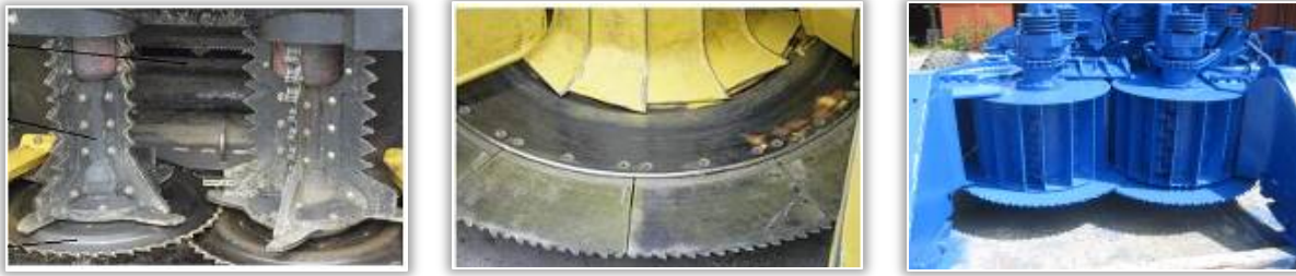
Figure 2 – Types of drums with cutting and pulling disk [13]
