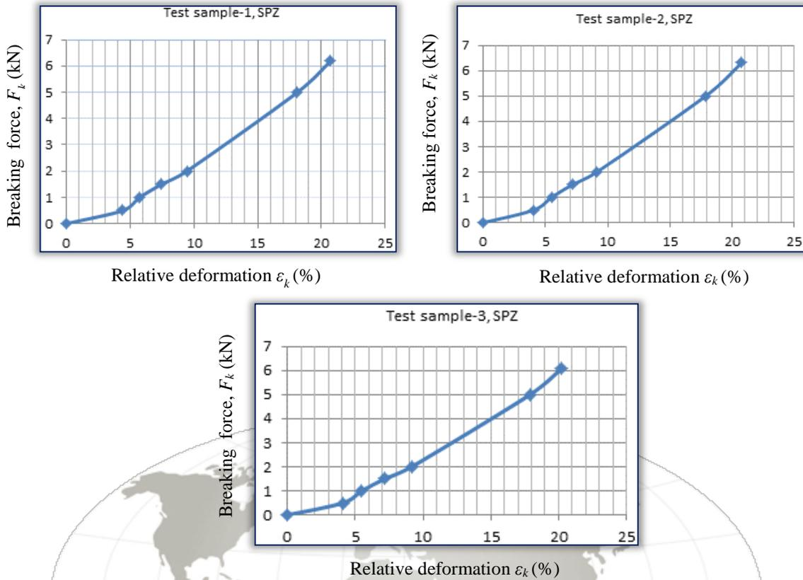
Figure 2. Force – relative deformation diagrams for SPZx737L<sub>p</sub>
