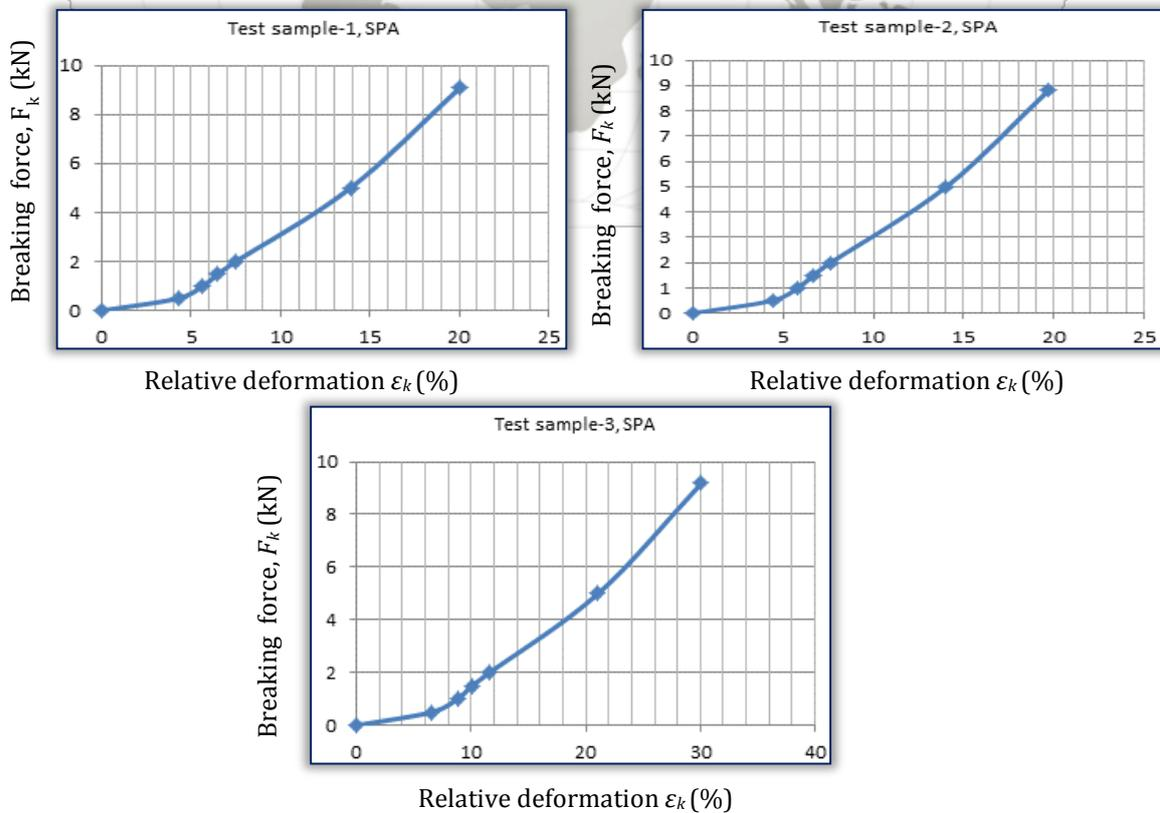
Figure 3. Force – relative deformation diagrams for SPAx982L<sub>p</sub>
