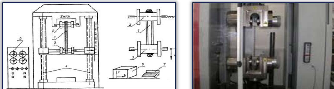
Figure 1. Tensile machine for investigation of belt characteristics: 1. Belt, 2. & 3. Pulleys, 4. Shaft with trapezoidal threads, 5. Remote control, 6. Computer, and 7. Keyboard
