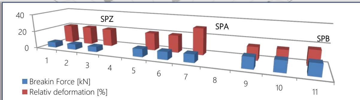
Figure 5. Graphical representation of the breaking force  $F_k$  [kN] and relative deformation  $\epsilon_k$  [%] for investigated samples
