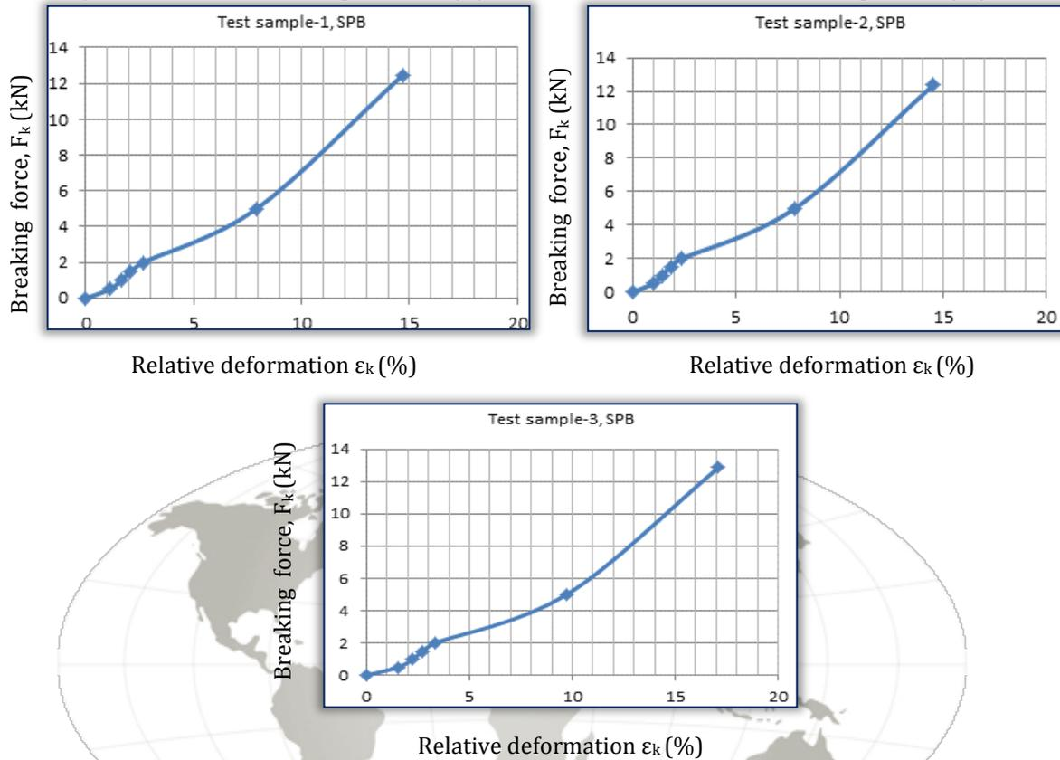
Figure 4. Force – relative deformation diagrams for SPBx2000L<sub>p</sub>
