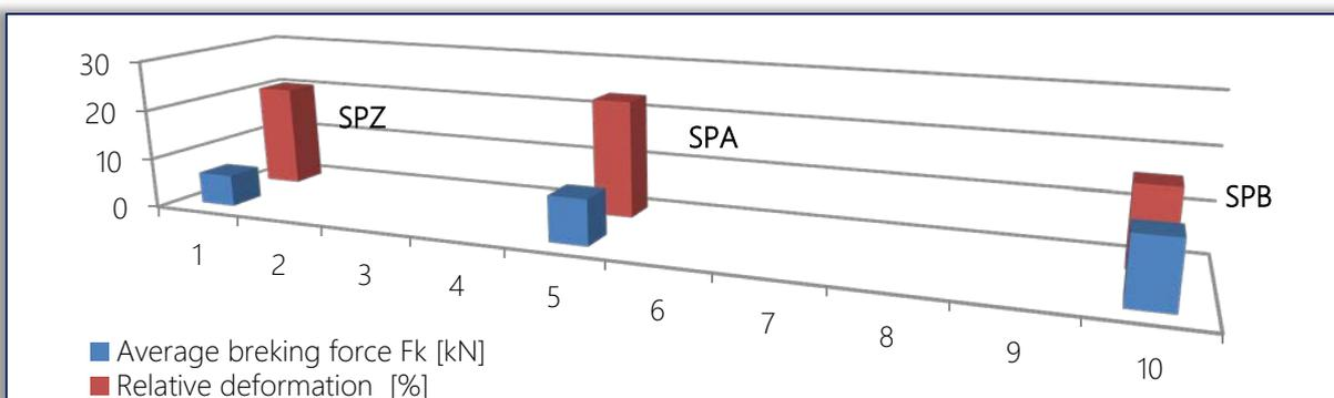
Figure 6. Graphical representation of the breaking force  $F_k$  [kN] and average relative deformation  $\epsilon_k$  [%] for investigated samples
