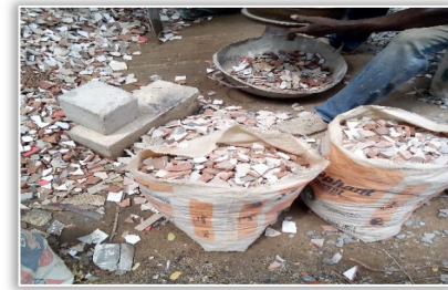
Figure 1- Crushing and Sieving of Ceramic Waste
