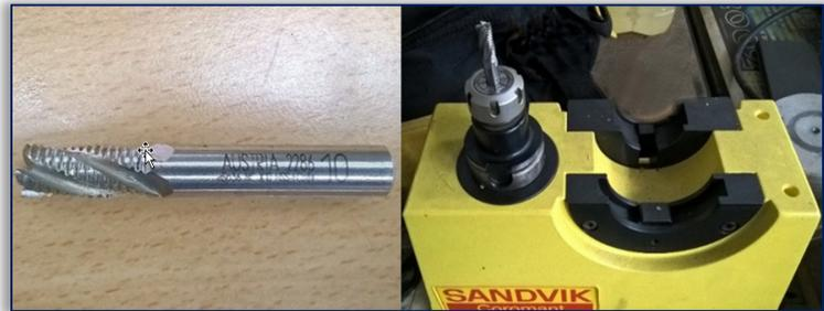
Figure 2. Tool and tool holder used for machining
