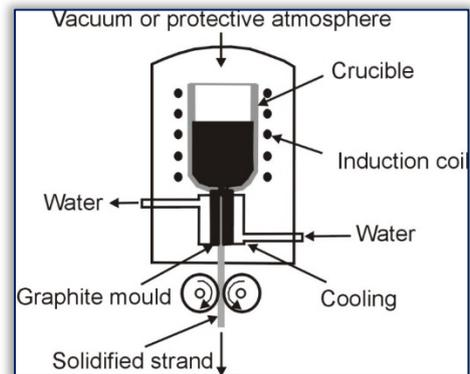
Figure 1. Schematic illustration of vertical continuous casting technology [7]
