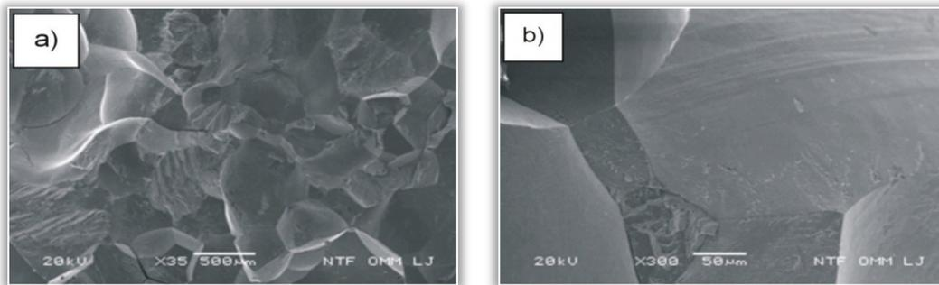
Figure 4. Microfractography of CuAlNi SMA after quenching at 850 °C/60'/WQ and tempering at 300 °C/60'/WQ; magnification: a – 35x, b – 300x
