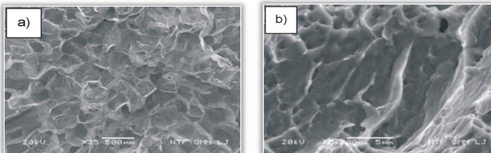
Figure 3. Microfractography of CuAlNi SMA after quenching at  $850 \text{ }^\circ\text{C}/60'/\text{WQ}$ ; magnification: a – 35x, b – 5000x
