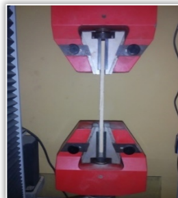
Figure 4: Tension Test arrangement
