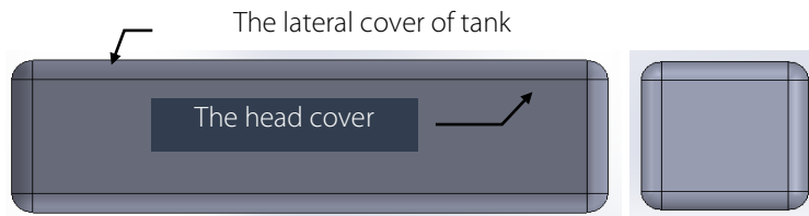
Figure 1. The geometrical model of pressurized parallelepipedic fuel tank
