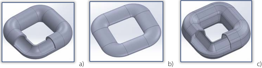
Figure 5. The axonometric representation of a sectioned toroidal surface generated by: a) C_G – circle and C_D - square; b) C_G – ellipse and C_D - square; c) C_G – septagon and C_D – square
