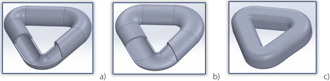
Figure 4. The axonometric representation of a sectioned toroidal surface generated by: a) C_G – circle and C_D - equilateral triangle; b) C_G – ellipse and C_D - equilateral triangle; c) C_G – square and C_D - equilateral triangle
