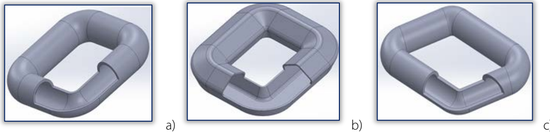
Figure 6. The axonometric representation of a sectioned toroidal surface generated by: a) C_G – circle and C_D - rectangle; b) C_G – pentagon and C_D - rectangle; c) C_G – ellipse and C_D – rectangle
