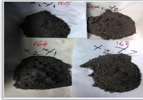
Figure 7. Precipitated brass powder after separation from the solubilization solution and after the drying operation
