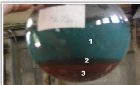
Figure 6. Precipitation of the solid phases in the acidic solution of CuSO 4 and ZnSO 4 . 1. Acid solution with Cu and Zn sulfate; 2. Precipitated neutral-sludge oxides
