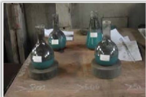
Figure 5. The four reagent vessels assembly after the second solubilization phase
