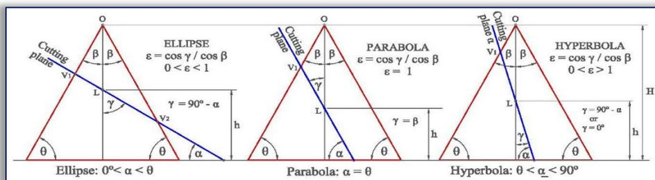
Figure 3. The main parameters used in geometrical constructions of conic sections
