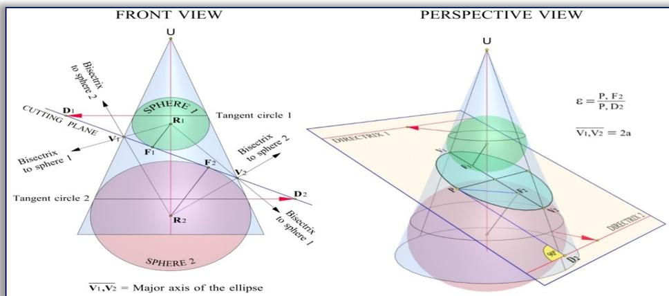
Figure 2. The components of an ellipse with the Dandelin spheres and the focus-directrix property
