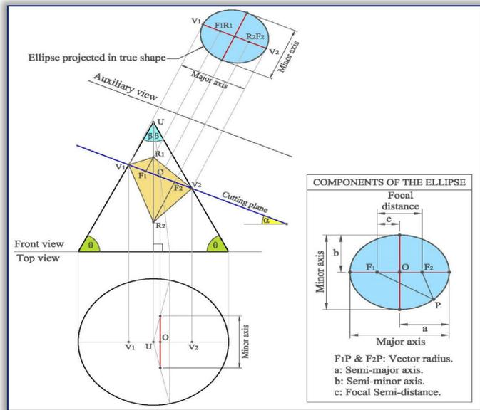
Figure 6. Projection of an ellipse in descriptive geometry and its components
