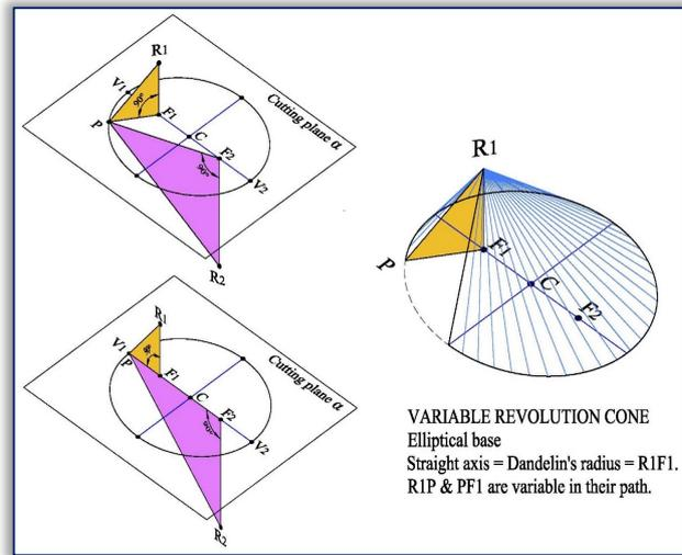
Figure 4. Right triangles orthogonal to the ellipse's plane
