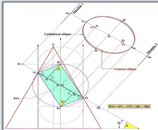
Figure 11. Comparison between a cylindrical and conical ellipse
