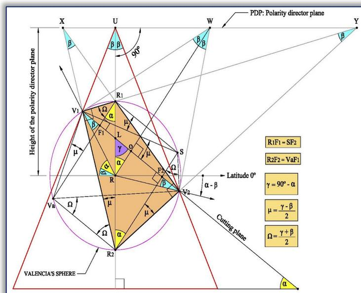
Figure 10. Graphical representations of convergence of the quadrilateral of Ptolemy, and tangency in the Valencia's sphere
