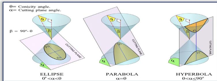
Figure 1. Conic sections
