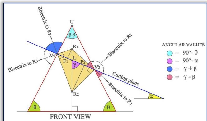
Figure 5. The front view of the right circular cone with its real and supplementary angles, and bisectrices
