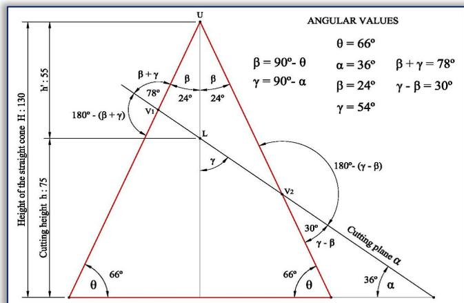
Figure 7. Geometrical constructions for a right circular cone with an elliptical section
