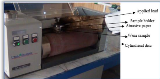
Figure 1. Pin on ring wear tester
