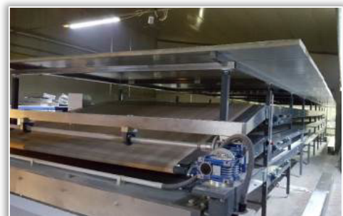
Figure 5 - Tunnel prover with three conveyors (source: Pani Enterprise Arges)
