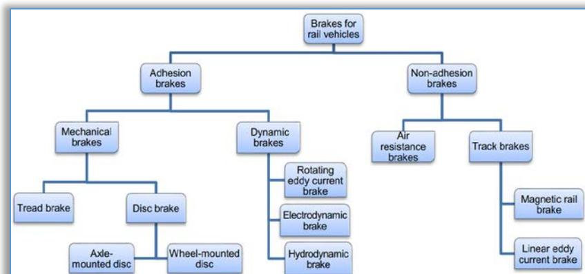
Figure 1. Types of brakes for rail vehicles [4]
