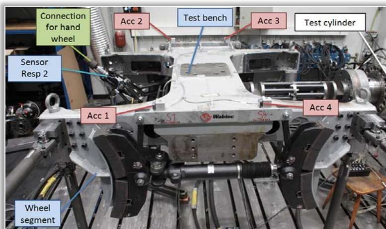
Figure 9. Photograph of vibration test bench and IBB 10 for longitudinal vibration and shock tests [7]
