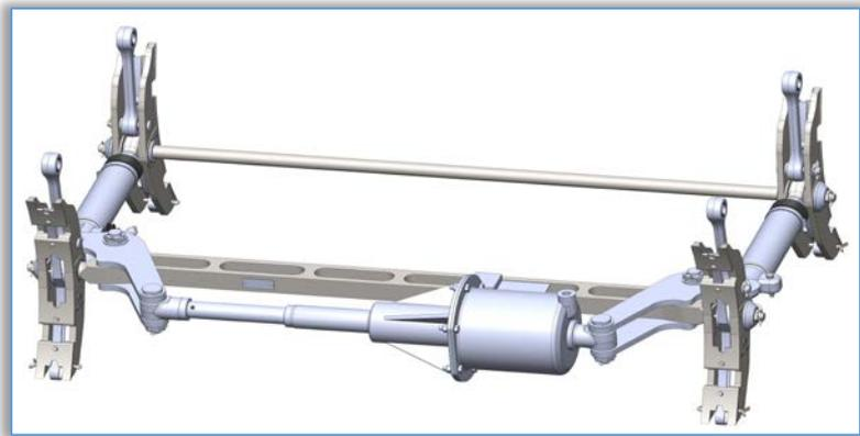
Figure 2. Model of innovative brake system IBB 10 without hand brake [10]
