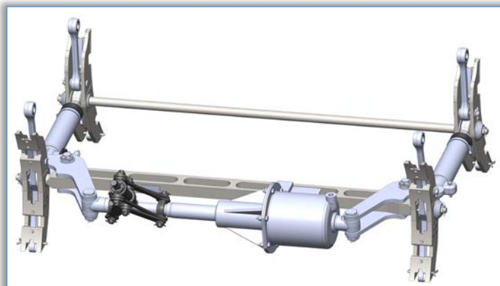
Figure 3. Model of innovative brake system IBB 10 with platform hand brake [10]
