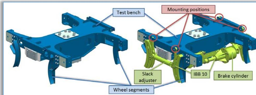
Figure 5. Schematic view of the vibration test bench with IBB 10 [7]
