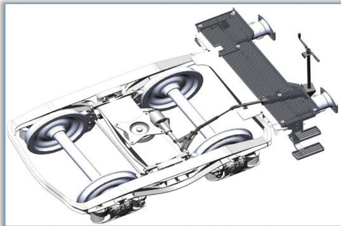
Figure 4. Model of Y25 bogie with installed brake system IBB 10 with platform hand brake and connection components for activation with segment of the wagon platform
