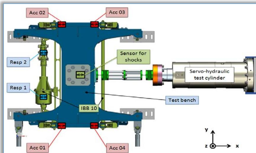
Figure 6. Schematic view of the vibration test bench with IBB 10 for longitudinal tests [7]
