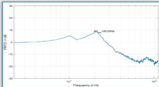
Figure 11. FRF diagram from vibration in vertical direction (z - direction) [7]
