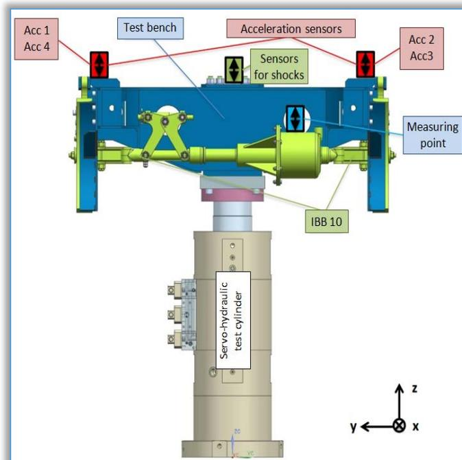
Figure 8. Schematic view of the vibration test bench with IBB 10 for vertical tests [7]
