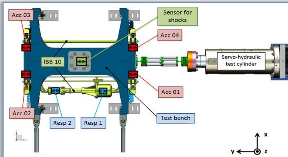
Figure 7. Schematic view of the vibration test bench with IBB 10 for side tests [7]
