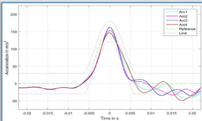
Figure 12. Acceleration diagram of vertical shock test [7]
