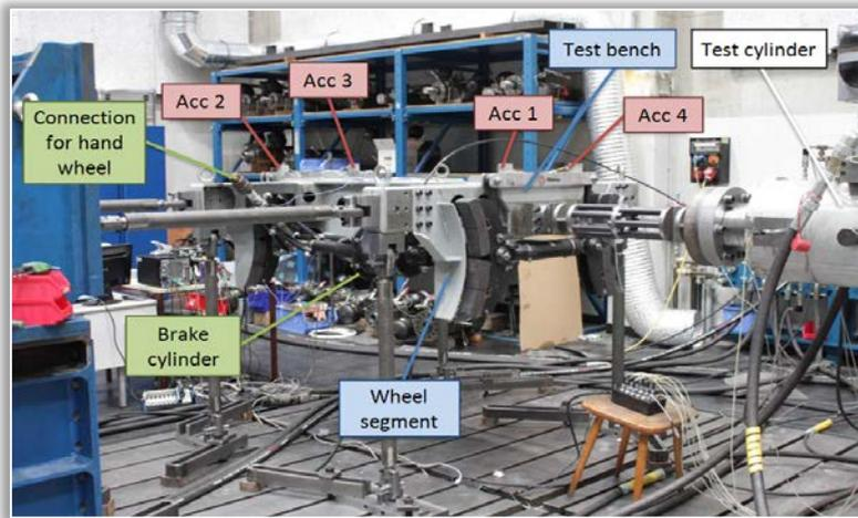
Figure 10. Photograph of vibration test bench and IBB 10 for side vibration and shock tests [7]
