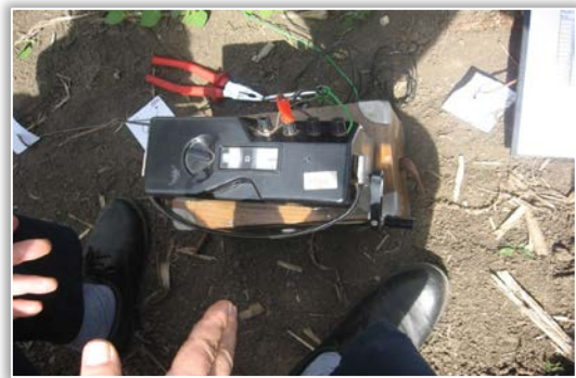
Figure 4. Instrument for the resistive bridge measuring method
