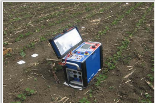
Figure 5. Instrument for the standard U-I measuring method
