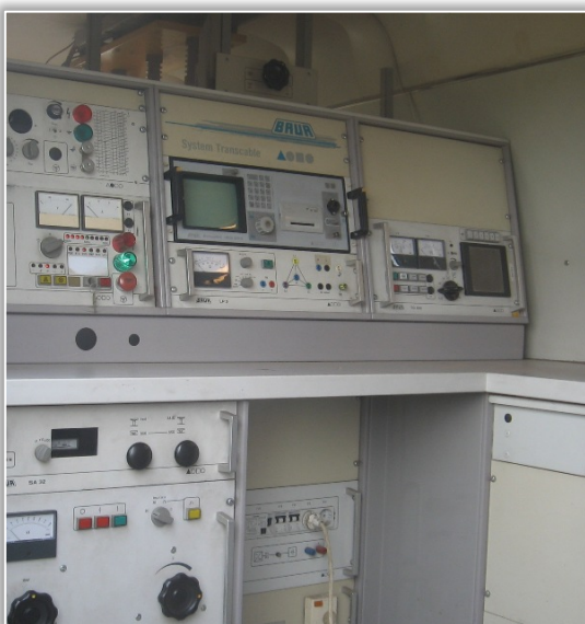
Figure 6. 230 V, AC source, positioned in the specialized van
