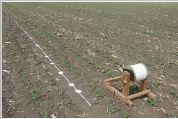
Figure 3. Prepared measuring path with the measuring probe sticks driven into the ground, at the predefined distances
