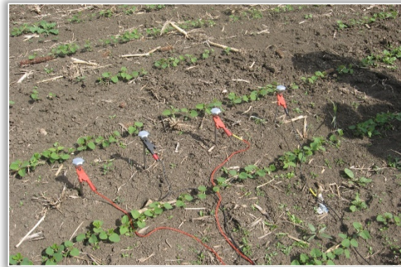
Figure 3. Prepared measuring path with the measuring probe sticks driven into the ground, at the predefined distances
