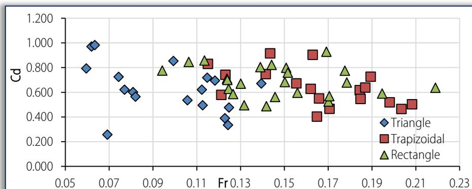
Figure 5. Variation of Coefficient of discharge with Upstream Froude Number
