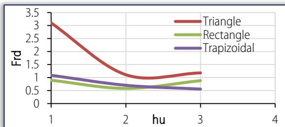
Figure 10. Variation of Downstream Froude Number with depth above weir for H=9cm, d=4cm
