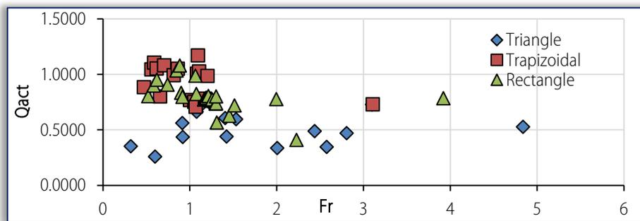
Figure 4. Variation of Measured Discharge with downstream Froude Number
