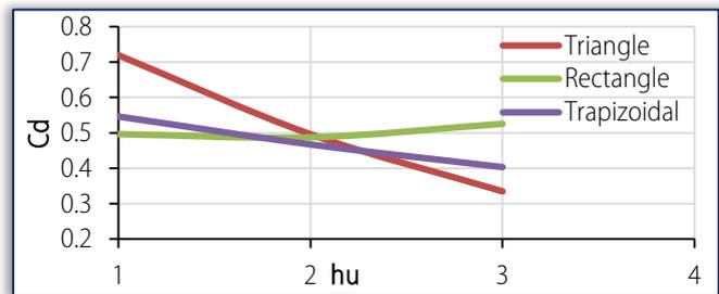
Figure 8. Variation of Discharge Coefficient with depth above weir for H=9cm, d=4cm
