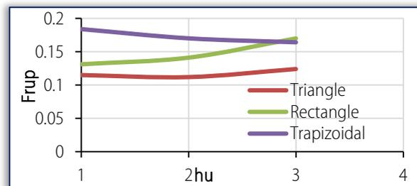
Figure 11. Variation of upstream Froude Number with depth above weir for H=9cm, d=4cm
