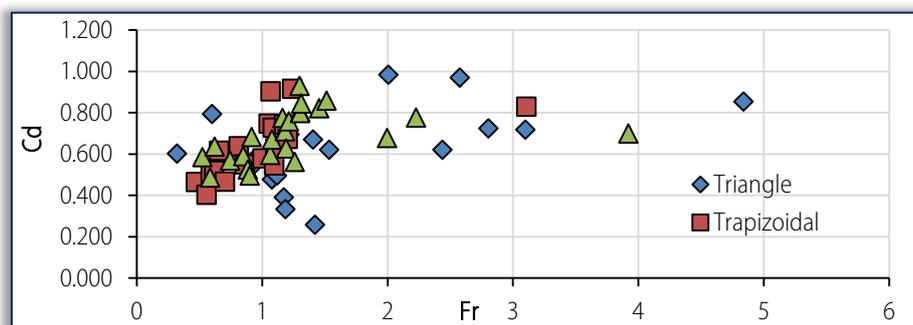
Figure 2. Variation of Coefficient of discharge with downstream Froude Number
