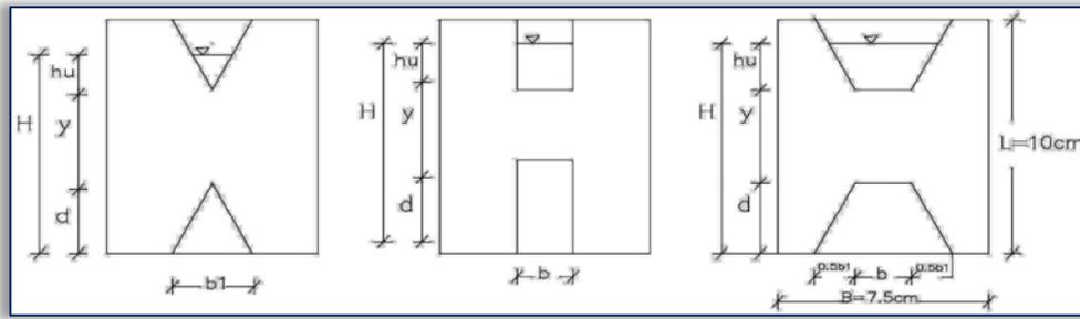
Figure 1. Definition Sketch for the Three Models of Combined Free Flow over Weir and under Gate
