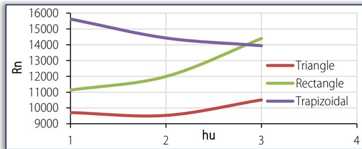
Figure 12. Variation of Reynolds Number with depth above weir for  $H=9\text{cm}$ ,  $d=4\text{cm}$
