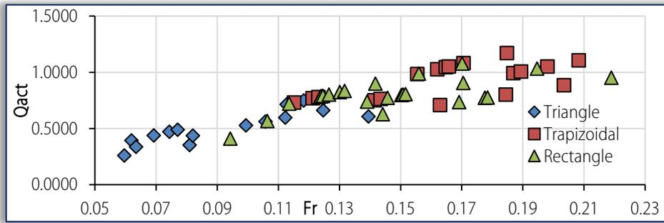
Figure 7. Variation of Measured Discharge with Upstream Froude Number
