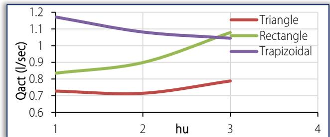
Figure 9. Variation of Measured Discharge with depth above weir for H=9cm, d=4cm
