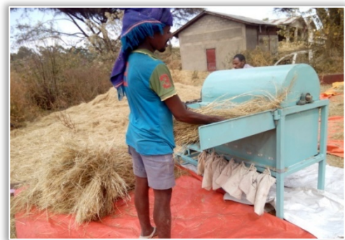
Figure 9. New developed threshing unit (manual feeding) under test
