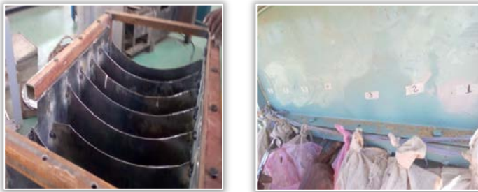
Figure 7. Sample (tef, straw and chaff mixture) collectors
