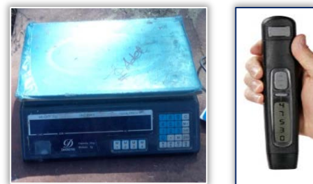
Figure 10. a) Sensitive balance for measuring samples weigh; b) Optical tachometer
