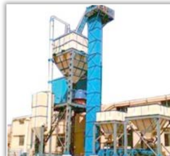
Figure 2 - Conveyor belts system from a compound feed factory consisting of horizontal conveyor belts (a) and vertical elevators (b)
