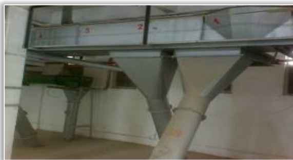
Figure 2 - Conveyor belts system from a compound feed factory consisting of horizontal conveyor belts (a) and vertical elevators (b)
