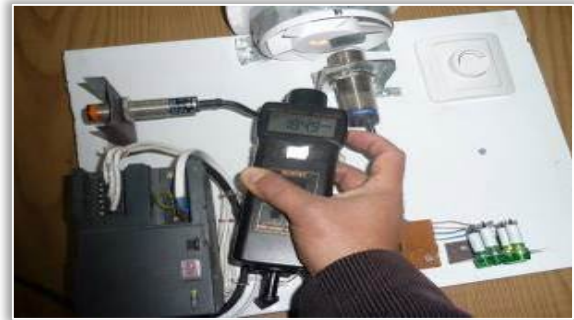
Figure 8 - Measuring the speed of rotation of the metallic lamella with the electronic tachometer
