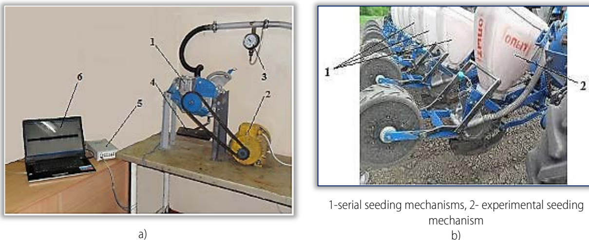
Figure 3 – General view of installation for tests in laboratory conditions (a) a seeding machine with experimental seeding section (b)
