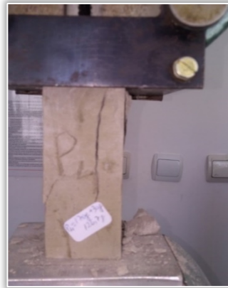
b) Prism test specimen being tested on the machine with cross-cracks
