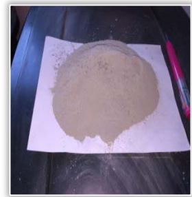
d) Slag with a granulation of 125µm
