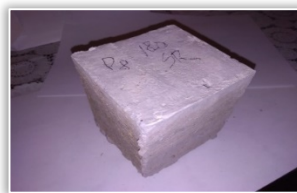
b) Cubic test specimens 7.07x7.07x7.07mm
