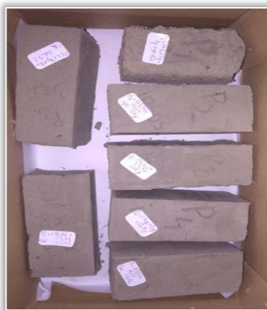
a) Prism test specimens of 40x40x100mm
