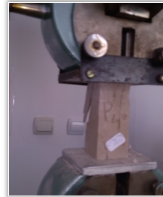
c) Prism test specimen being tested on the machine with splitting cracks
