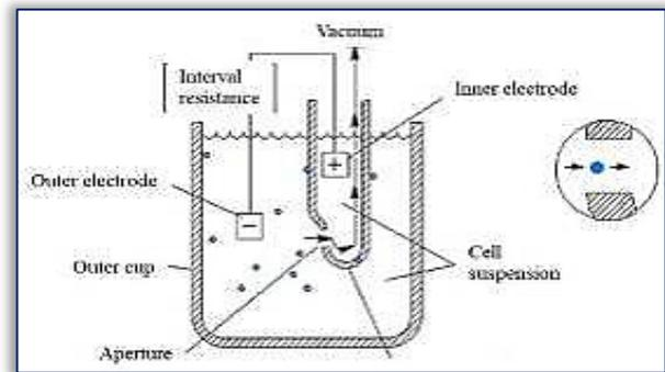
Figure 5 - Electrical resistance working diagram
