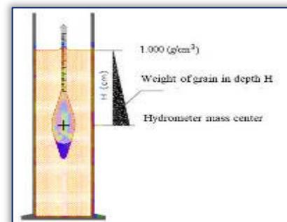
Figure 6 - Hydrometer measurement technique
