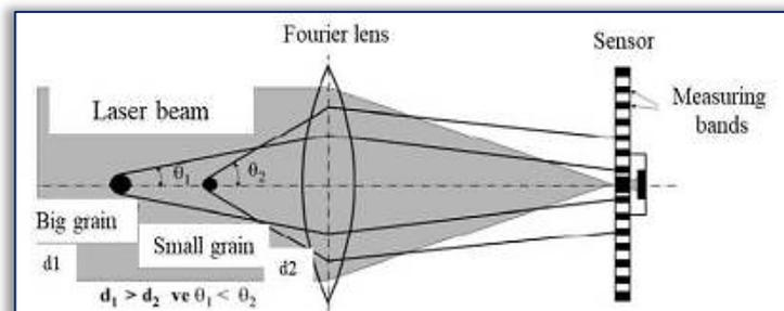
Figure 3 - Inversely proportional relationship between the size of the grains and the angle of refraction of the rays
