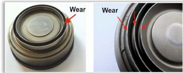
Figure 1. Examples of compression mould with signs of wear
