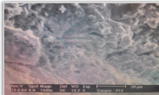
Plate 2: SEM for concrete with 10% NSHA
