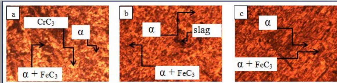
Plate 3. Micrograph of the (a) weldment; (b) HAZ; (c) base metal of 60° bevel angle after etched in 2% Nital solution at magnification 100x
