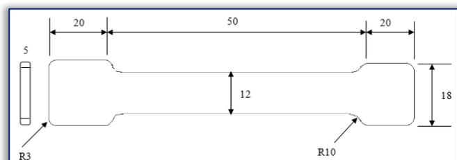
Figure 1: Tensile Strength Sample Schematic Drawing
