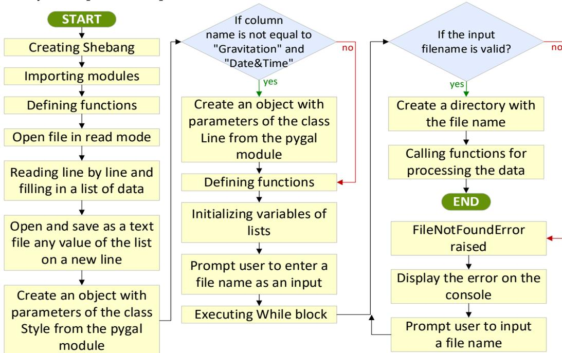
Figure 7. Algorithmic diagram of the CHARTS\_PYGAL program
