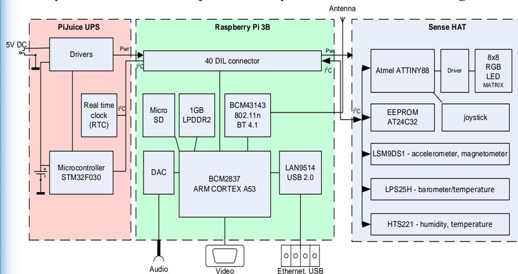
Figure 1. Structure diagram of the system
