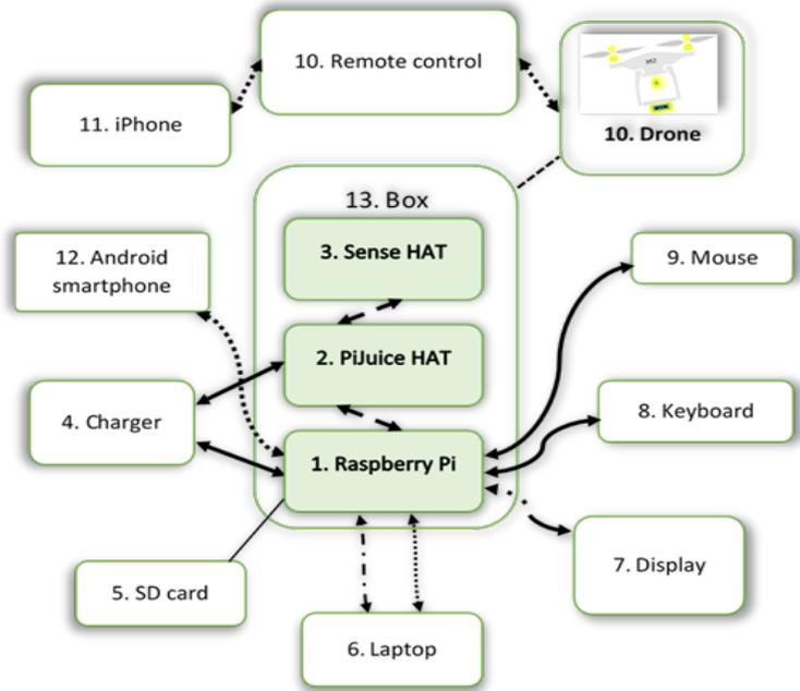
Figure 2. Functional diagram of the system
