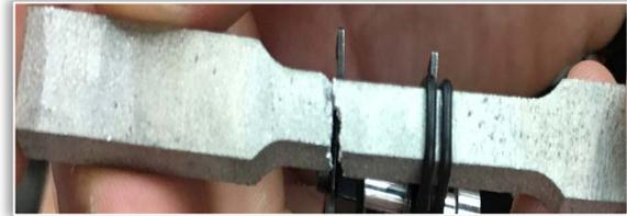
Figure 5. Specimens after testing
