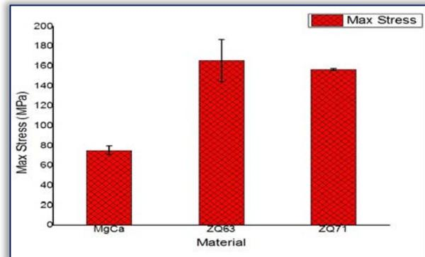
Figure 7. Maximum stress compared to the three types of magnesium alloys studied
