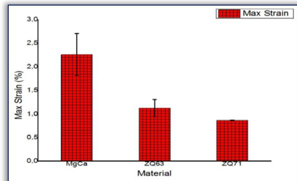
Figure 8. Maximum strain compared to the three types of magnesium alloys studied
