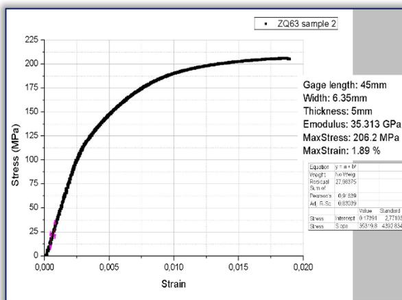
Figure 2. Stress–strain curve for ZQ63 alloys
