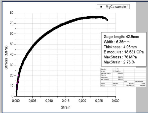
Figure 4. Stress-strain curve for MgCa alloys
