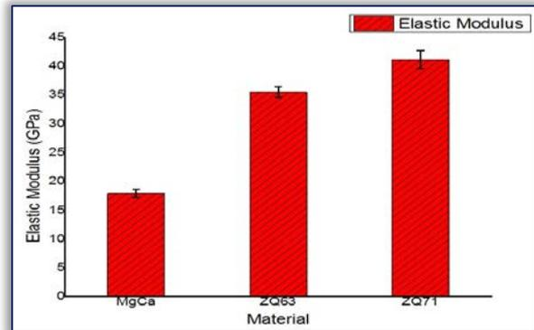
Figure 6. Elastic modulus compared to the three types of magnesium alloys studied
