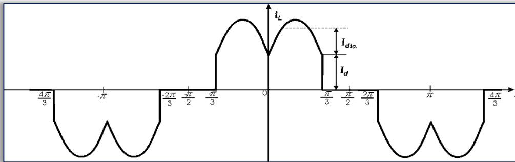
Figure 5. Flow of the filament current  $i_L$  of the three phase bridge rectifier with a load greater than  $I_{d\alpha}$  and with the thyristor commutation effect neglected
