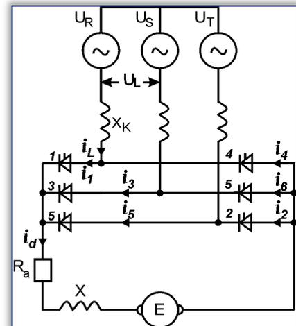
Figure 2. Scheme of the three phase bridge rectifier with reduced parameters of the rectifying transformer and the network at the secondary end of the rectifying transformer
