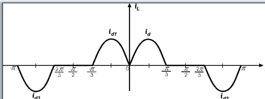
Figure 3. Flow of the current  $i_L$  of the three phase bridge rectifier with the load at the intermittent current limit
