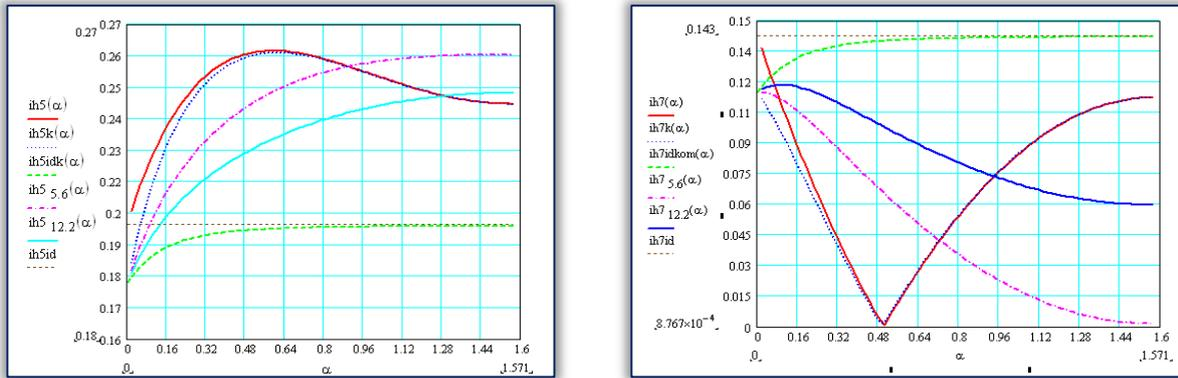
Figure 6. Flows of the relative values of the harmonics of current of 5., 7., ranges at the network end of the three phase bridge rectifier in the function of the thyristor ignition angle, the various parameters of  $u_k=0.05$  and the relationship of  $X / X_K=(1.6.,5.6.,12.2.)$
