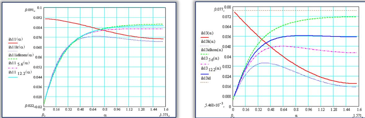
Figure 7. Flows of the relative values of the harmonics of current of 11., 13., ranges at the network end of the three phase bridge rectifier in the function of the thyristor ignition angle, the various parameters of  $u_k=0.05$  and the relationship of  $X / X_K=(1.6.,5.6.,12.2.)$
