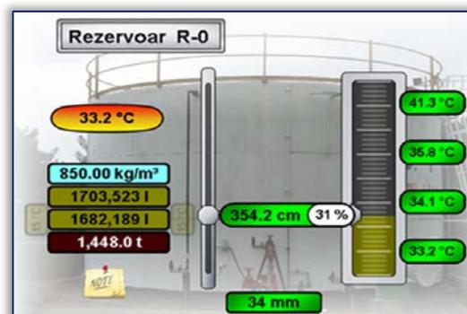
Figure 3. SCADA screen for displaying measured values, displaying alarms and simulated values
