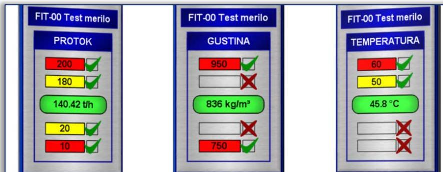
Figure 9. SCADA screen for Adjusting flow, density and temperature
