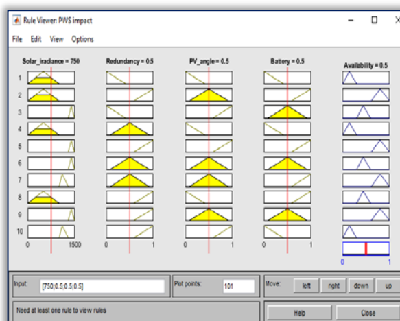
Figure 7. Generation of the decision surface (a) and the inference graphs (b,) for analyzing the availability of electricity from the photovoltaic power plant
