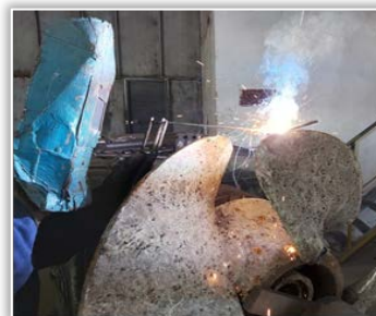
Figure 8. Welded piece added
