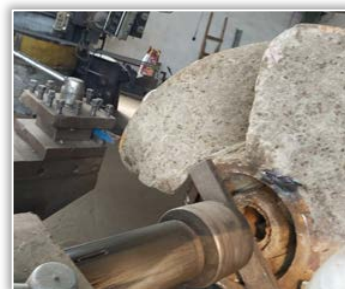
Figure 6. Rotor machined by cutting on the lathe
