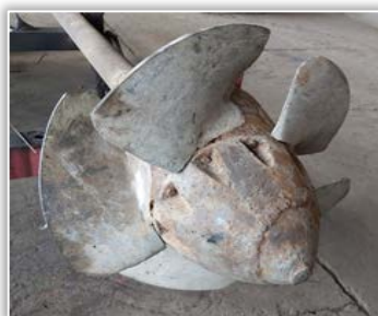
Figure 5. Pump rotor requiring blade replacement
