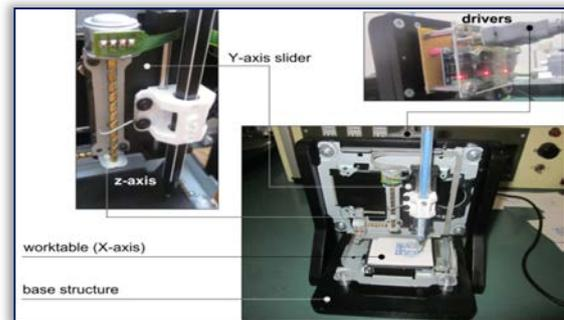
Figure 10. Fully integrated mechanical and control hardware
