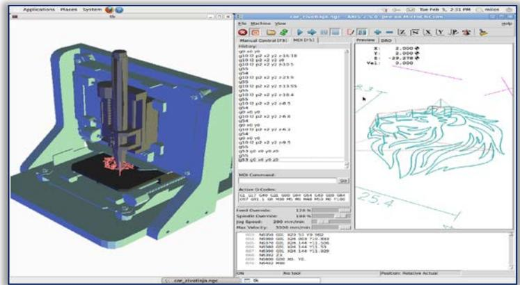
Figure 9. The Virtual machine integrated with the graphic user interface AXIS
