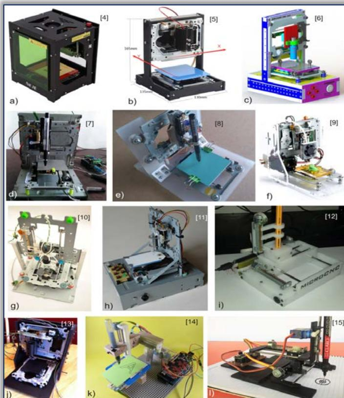
Figure 1. Mini CNC machine tools based on CD/DVD drive hardware [4–15]
