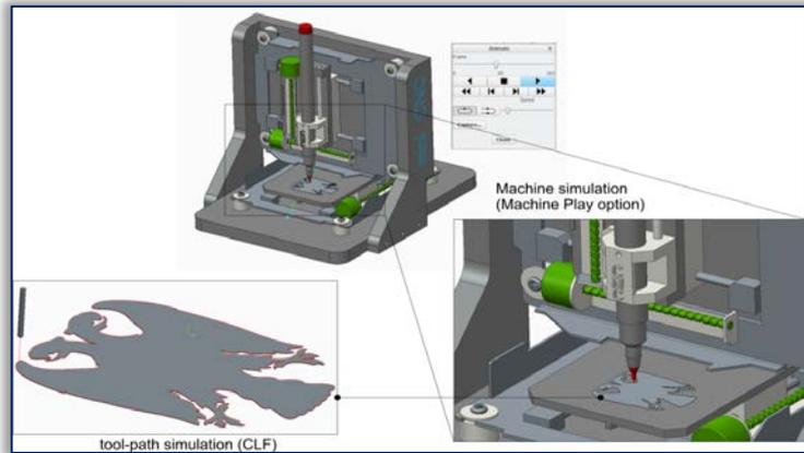
Figure 4. Example of the simulation within the CAD/CAM environment with active virtual machine executing the given machining program (CLF)
