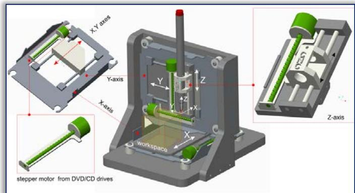
Figure 2. CAD model of the table 3-axis mini CNC machine tool with basic components
