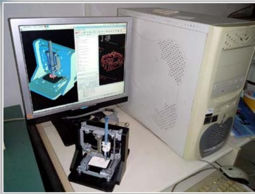
Figure 12. Machine work environment with PC control system and integrated virtual machine in the background
