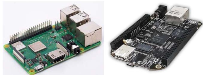
Figure 8. The compact PC platforms Raspberry Pi 3 Model B+ in BeagleBone black
