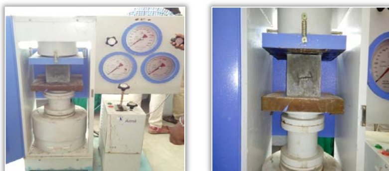
Figure 8. Compression Strength Testing Setup
