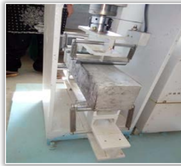
Figure 9. Flexural Strength Testing Setup
