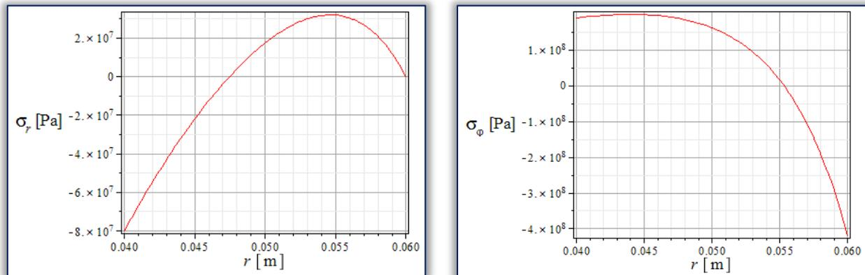
Figure 6. The radial and tangential normal stresses of the second numerical example
