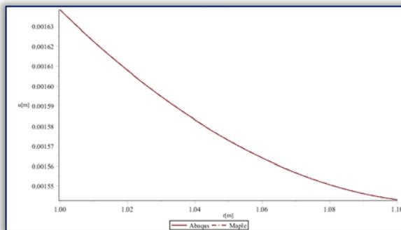
Figure 3. The displacement fields of the analytical and numerical methods
