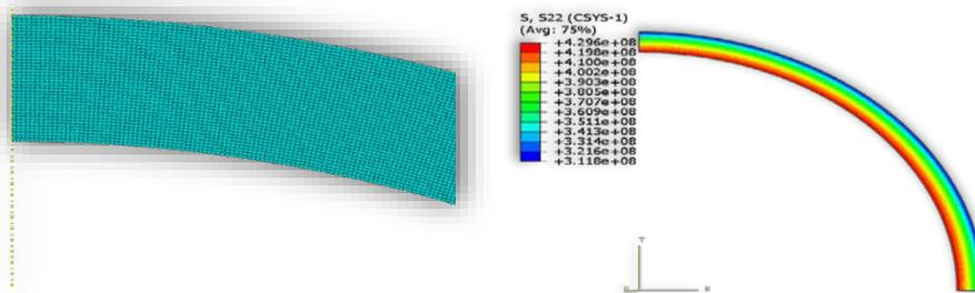
Figure 2. The finite element model of the sphere with the hoop stress
