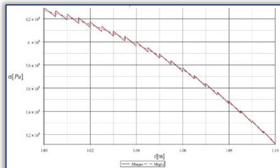
Figure 5. The hoop stresses coming from the finite element simulations and the analytical solution
