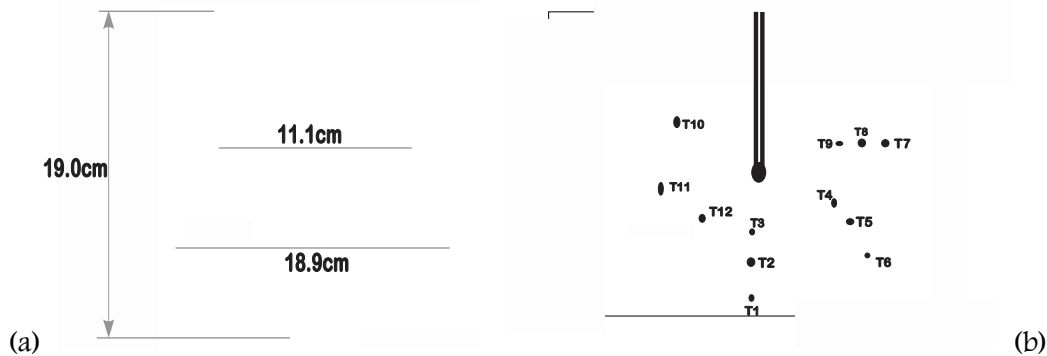
Figure 1: (a) Specification of the Zeer Pot used (b) Experimental set up
