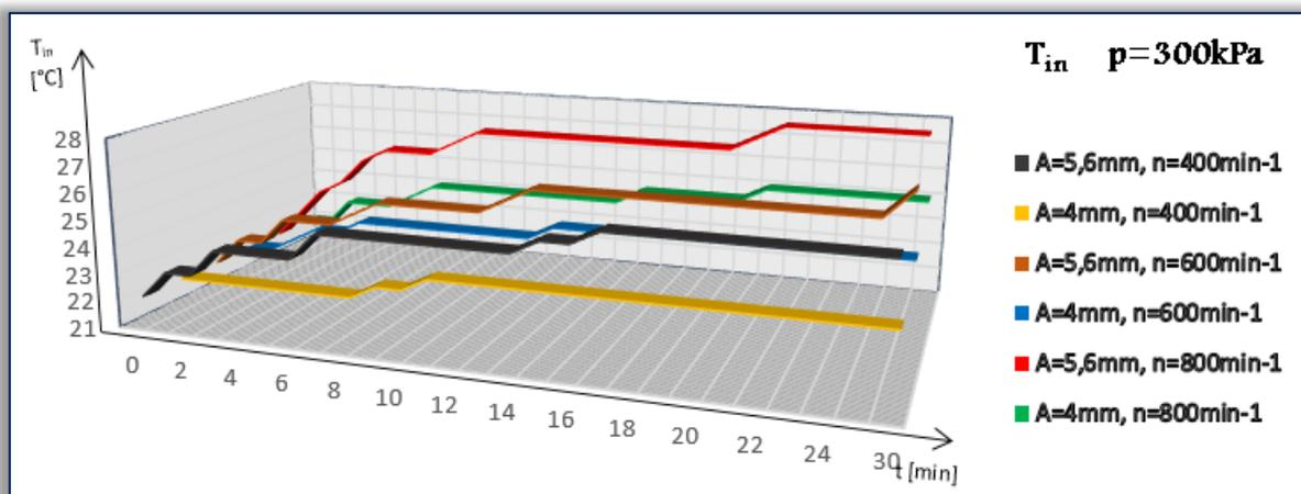
Figure 2. Comparison of measured the temperature inside the elastic element  $T_{in}$  at constant pressure  $p = 300\text{kPa}$  amplitude  $A = 4\text{mm}$  and  $A = 5.6\text{mm}$  at three different revolutions  $n=400\text{min}^{-1}$ ,  $n=600\text{min}^{-1}$  and  $n=800\text{min}^{-1}$ .
