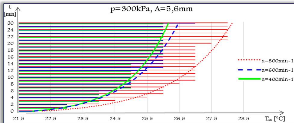
Figure 4 Comparison of measured development values the temperature inside the elastic element  $T_{in}$  for speed  $n = 400, 600, 800 \text{ min}^{-1}$  constant pressure  $p = 300\text{kPa}$  amplitude  $A = 5,6 \text{ mm}$ .
