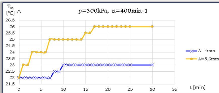
Figure 5. Comparison of measured values temperature inside the elastic element  $T_{in}$  for amplitudes  $A = 4$  and  $5,6\text{mm}$  at speed  $n = 400 \text{ min}^{-1}$  and constant pressure  $p = 300\text{kPa}$ .
