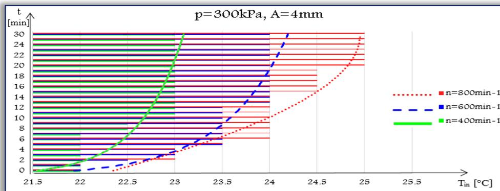
Figure 3. Comparison of measured development values temperature inside the elastic element  $T_{in}$  for speed  $n = 400, 600$  and  $800 \text{ min}^{-1}$  constant pressure  $p = 300\text{kPa}$  amplitude  $A = 4\text{mm}$ .
