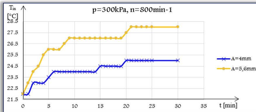
Figure 7. Comparison of measured values temperature inside the elastic element  $T_{in}$  for amplitudes  $A = 4$  and  $5,6\text{mm}$  at speed  $n = 400\text{ min}^{-1}$  and constant pressure  $p = 300\text{kPa}$ .
