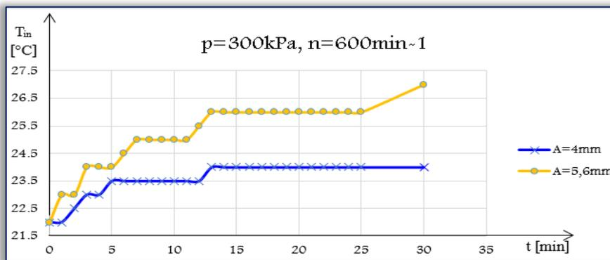
Figure 6. Comparison of measured values temperature inside the elastic element  $T_{in}$  for amplitudes  $A = 4$  and  $5.6\text{mm}$  at speed  $n = 600 \text{ min}^{-1}$  and constant pressure  $p = 300\text{kPa}$ .
