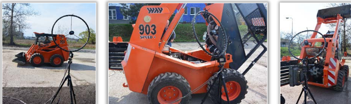
Figure 1. Wheel loader and installed acoustic camera
