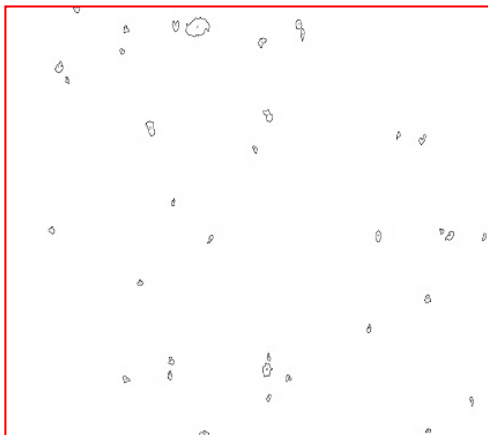
Fig.3a: Spheroidal Graphite Particles for Alloy C
