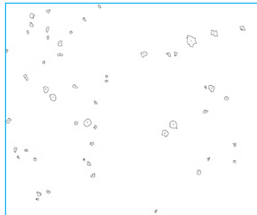
Fig.3b: Spheroidal Graphite Particles for Alloy A1
