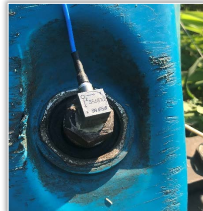
Figure 2. Accelerometer mounting positions – left handlebar, right handlebar, cutterbar
