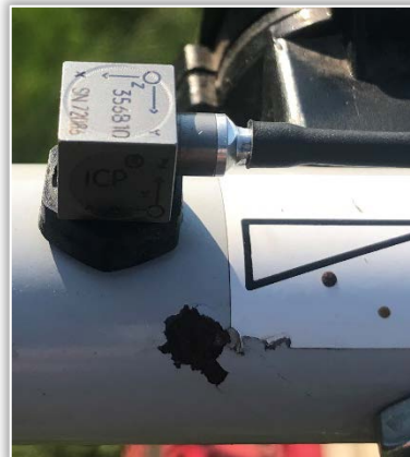
Figure 2. Accelerometer mounting positions – left handlebar, right handlebar, cutterbar
