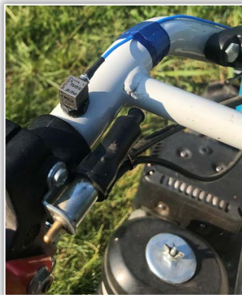
Figure 2. Accelerometer mounting positions – left handlebar, right handlebar, cutterbar
