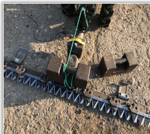
Figure 7. Auxiliary weights placement on the sickle bar
