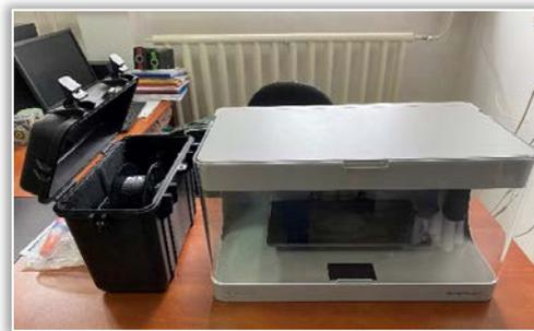
Figure 2. Markforged Onyx One 3D printer
