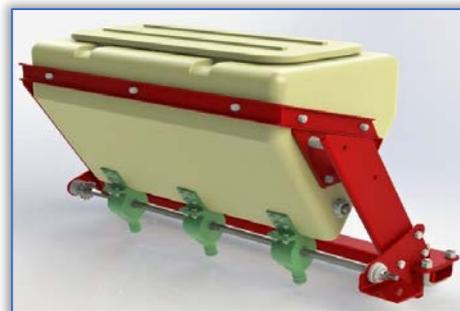
Figure 1. Box with grooved roll type dispenser
