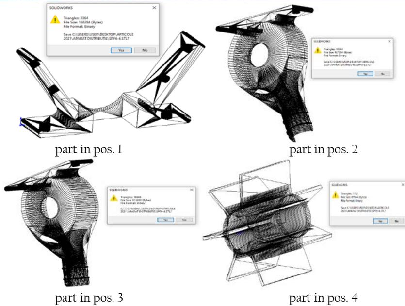
Figure 5. Saving the geometry of the dispenser's components in STL format
