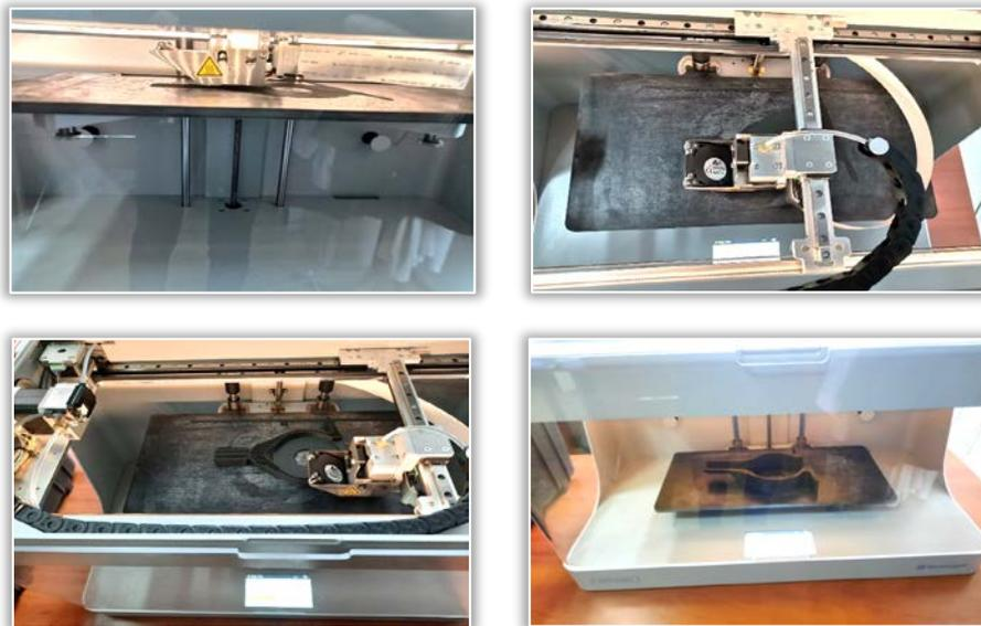
Figure 7. Different steps of 3D printing of the dispenser's components
