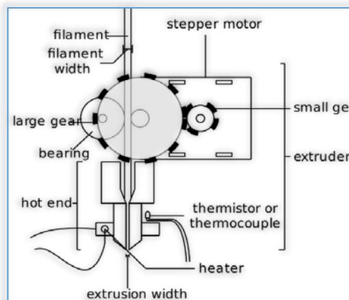
Figure 3. Technology used by Markforged Onyx One 3D printer [9]
