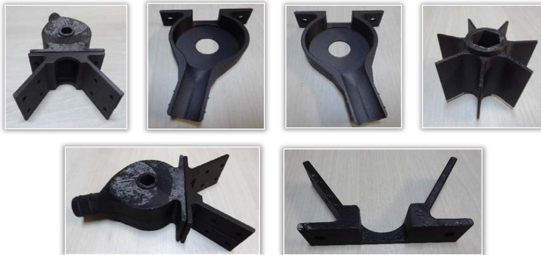
Figure 8. Dispenser and its components in the final version
