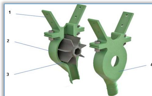
Figure 4. 3D CAD geometric model of the grooved roll type dispenser; 1–support, 2–left housing, 3– grooved roll, 4–right housing
