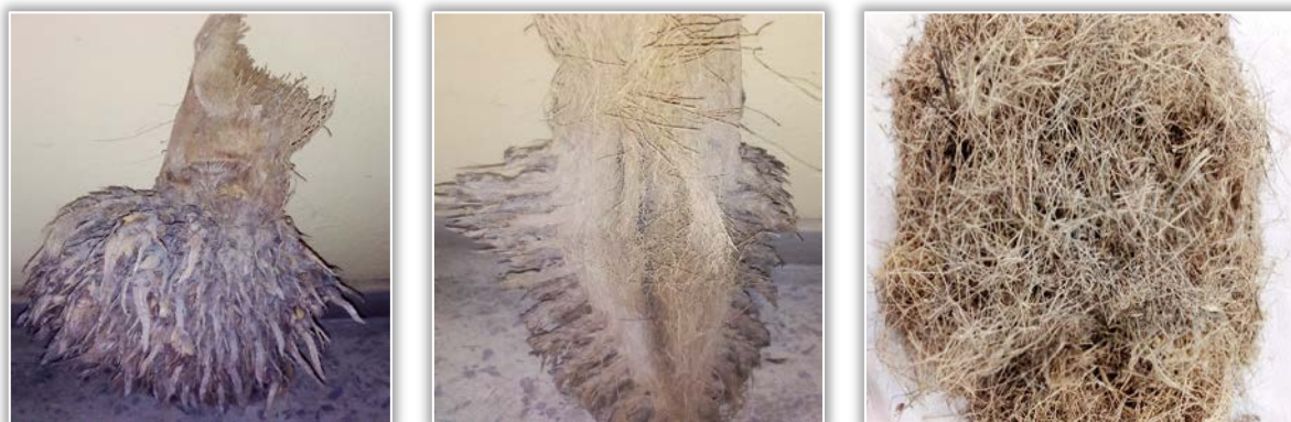
Figure 2: Oil palm empty fruit bunch fibres (OPE-FBF): (a) the Oil palm empty fruit bunch, (b) the fibre before extraction and (c) the fibres after extraction
