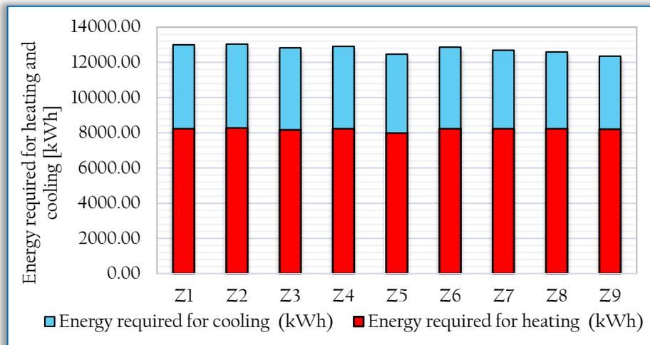
Figure 3. Total annual energy required for heating and cooling for MODEL III SI for different vegetation subvariants (Z1-Z9) and for WWR=20%
