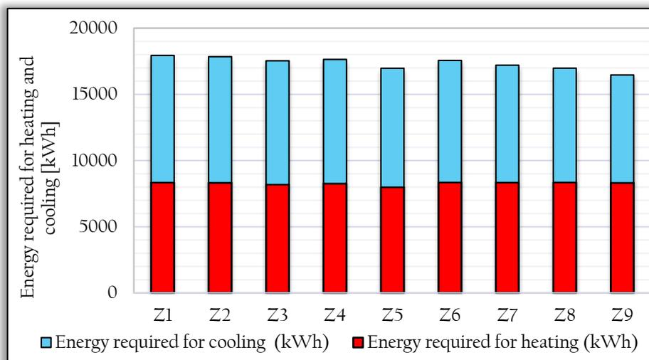
Figure 4. Total annual energy required for heating and cooling for MODEL III S1 for different vegetation subvariants (Z1-Z9) and for WWR=40%
