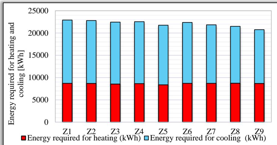
Figure 5. Total annual energy required for heating and cooling for MODEL III S1 for different vegetation subvariants (Z1-Z9) and for WWR=60%
