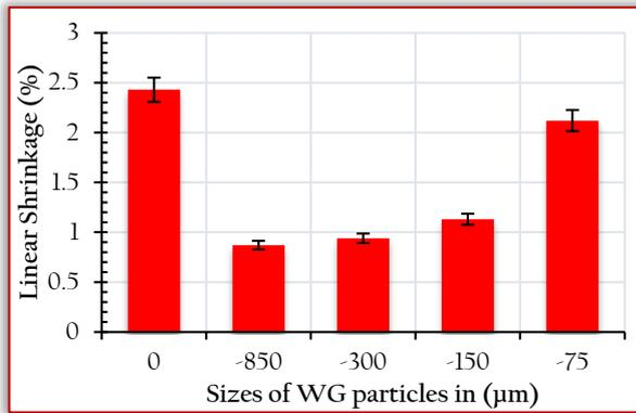
Figure 3: Effect of particle sizes on the Firing shrinkage of Fired Bricks
