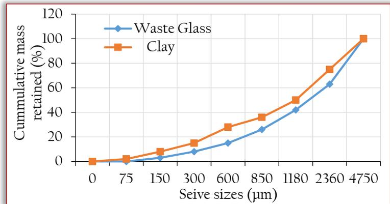
Figure 2: Particle Size Distribution of waste glass and clay
