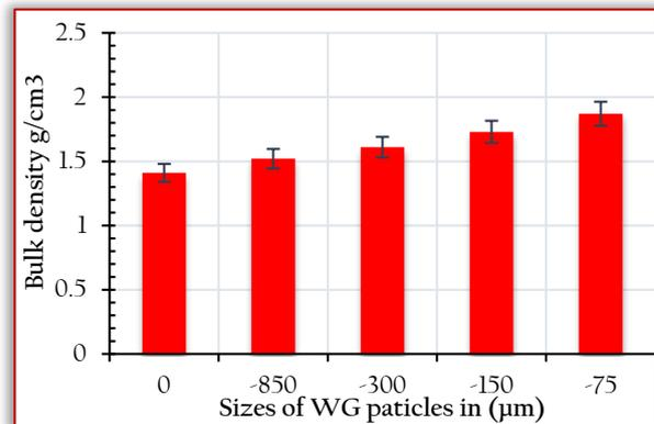
Figure 6: Effect of particle sizes on the Bulk Density
