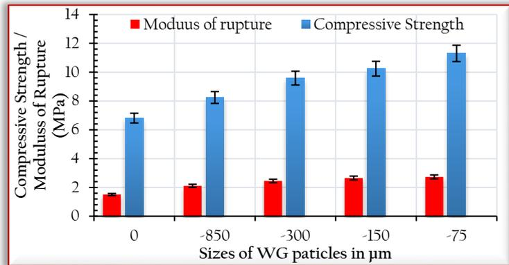
Figure 7: Effect of particle sizes on the Compressive Strength and Modulus of rupture
