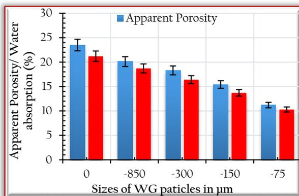
Figure 5: Effect of particle sizes on the Apparent Porosity and Water Absorption
