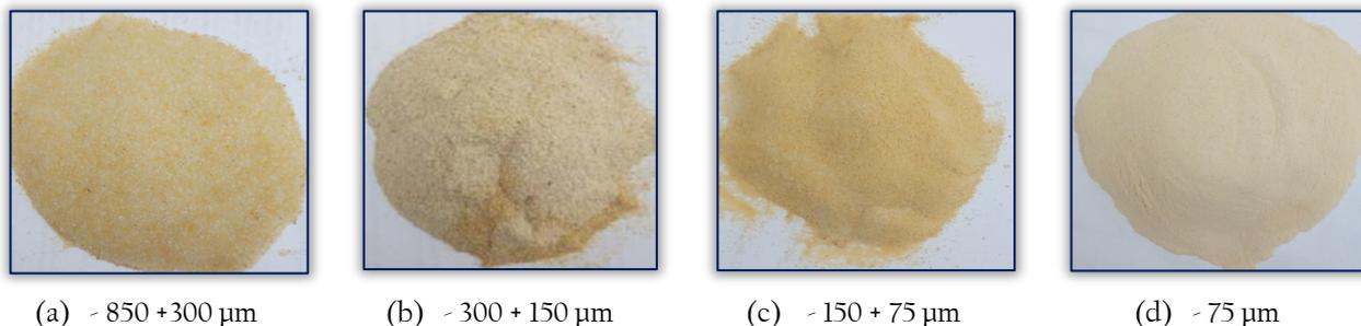
Figure 1: Particle sizes of waste glass particles employed in this study
