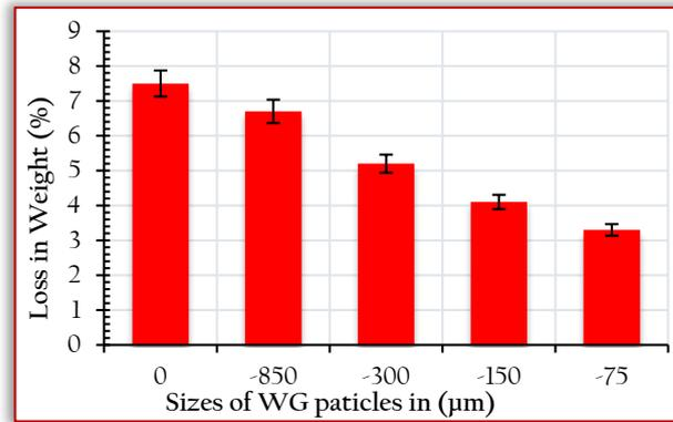
Figure 4: Effect of particle sizes on the weight loss of fired bricks
