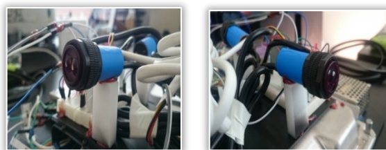
Figure 11. E18-D80NK left / right sensors located on the V2V / V2I test bench
