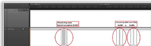
Figure 4. Answer received from the ECU with the sync byte, KW1 and KW2 (10400 baud)
