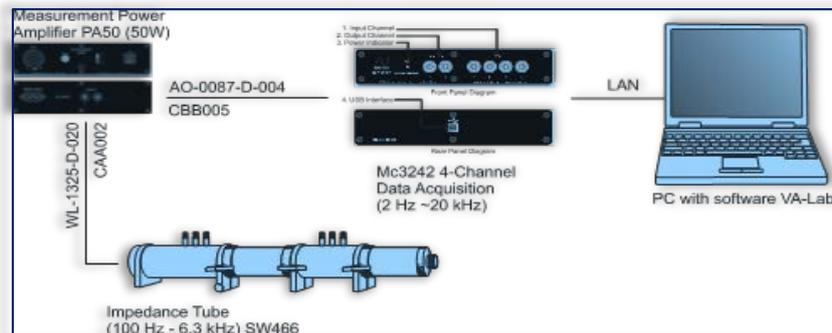
Figure 3. Wiring diagram of measuring technique for measuring the sound absorption factor  $\alpha$  (-)
