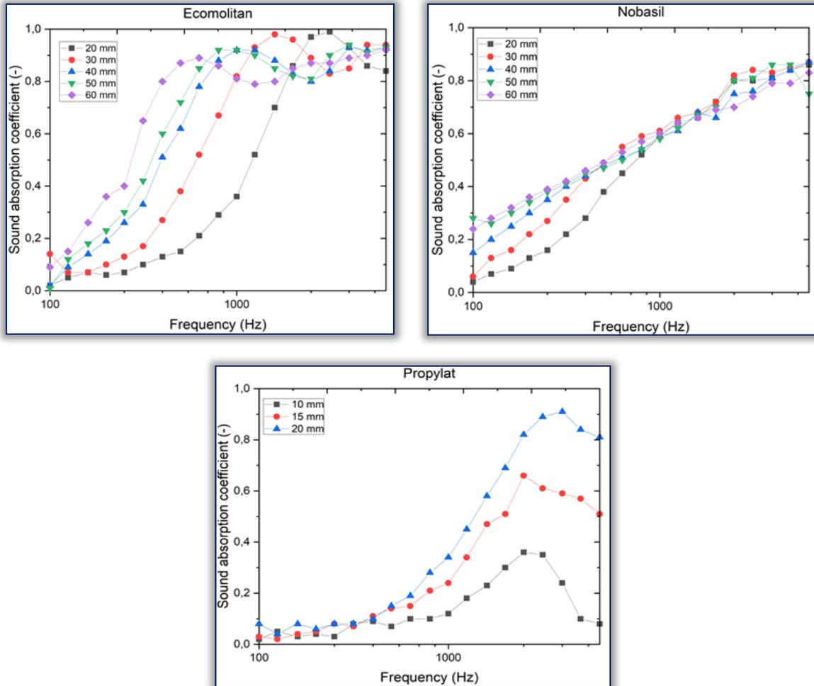
Figure 4. Demonstration of sound absorption coefficient values  $\alpha$  (-) for single-layer materials
