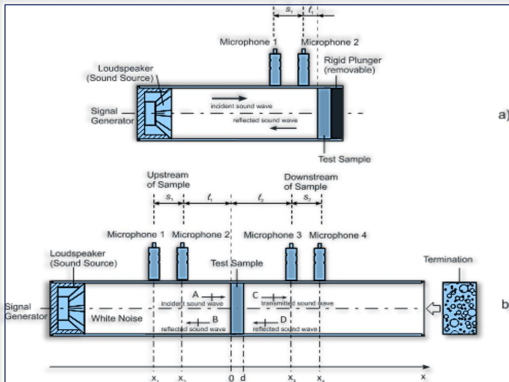
Figure 2. Schematic of the SW466 impedance tube, a) transmission method with two microphones, b) transmission method with four microphones
