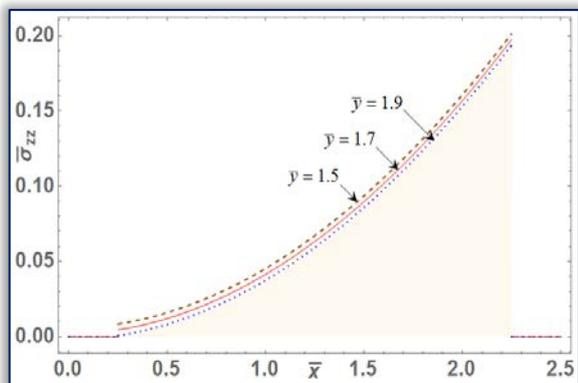
Figure 4 (d): Thermal stresses  $\bar{\sigma}_{zz}$  along  $\bar{x}$  – direction for different values of  $\bar{y}$ .
