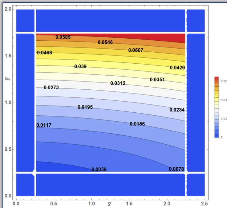
Figure 3 (d): Contour plot of deflection along  $\bar{x} - \bar{y}$  – plane for a fixed value of  $\tau$ .
