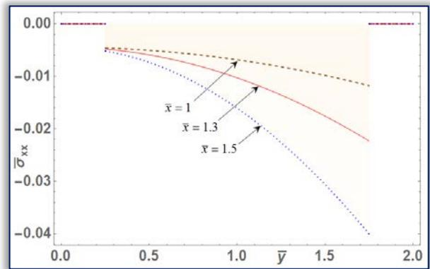
Figure 4 (b): Thermal stresses  $\bar{\sigma}_{xx}$  along  $\bar{y}$  – direction for different values of  $\bar{x}$ .
