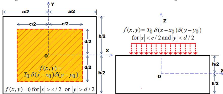
Figure 1. Schematic geometry of thick rectangular plate
