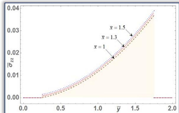
Figure 4 (e): Thermal stresses  $\bar{\sigma}_{zz}$  along  $\bar{y}$  – direction for different values of  $\bar{x}$ .
