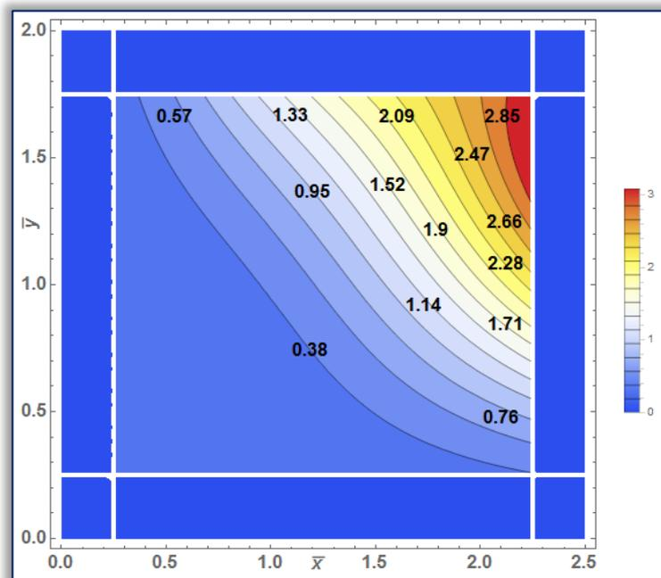
Figure 2 (d): Contour plot of temperature distribution along  $\bar{x} \bar{y}$  - plane for a fixed value of  $\bar{z}$ .
