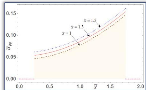
Figure 4 (c): Thermal stresses  $\bar{\sigma}_{yy}$  along  $\bar{y}$  – direction for different values of  $\bar{x}$ .
