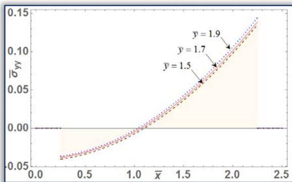
Figure 4 (b): Thermal stresses  $\bar{\sigma}_{yy}$  along  $\bar{x}$  – direction for different values of  $\bar{y}$ .
