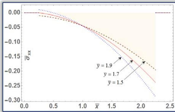
Figure 4 (a): Thermal stresses  $\bar{\sigma}_{xx}$  along  $\bar{x}$  – direction for different values of  $\bar{y}$ .
