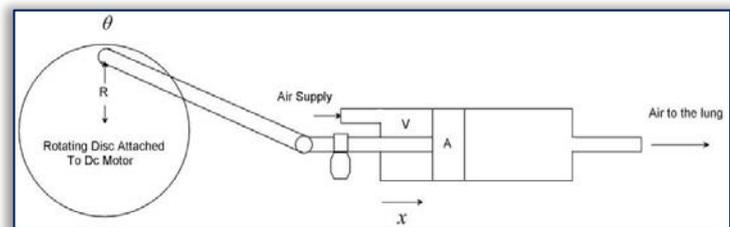
Figure 1. Respiratory ventilator system design
