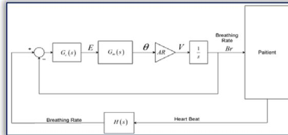
Figure 3. Closed loop system block diagram
