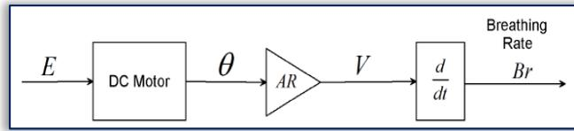
Figure 2. Block diagram of the ventilator
