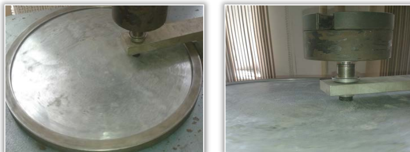
Figure 5. Test of abrasive wear on the steel plate of the test-pieces
