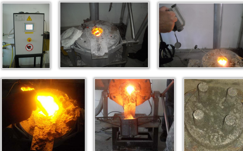
Figure 4. Preparation and casting of cast iron samples
