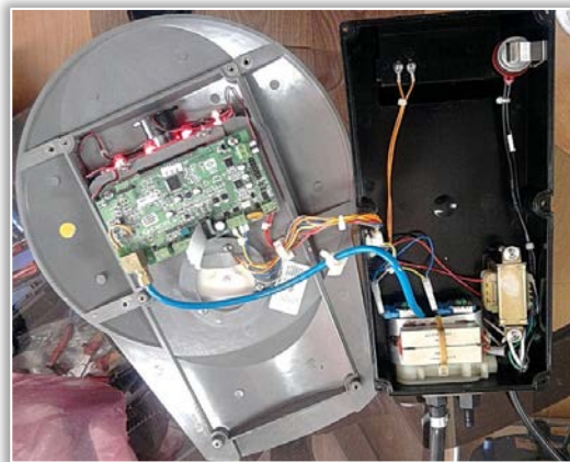
Figure 4. The appearance of the disassembled device for automatic pressure adjustment in car tires [11]
