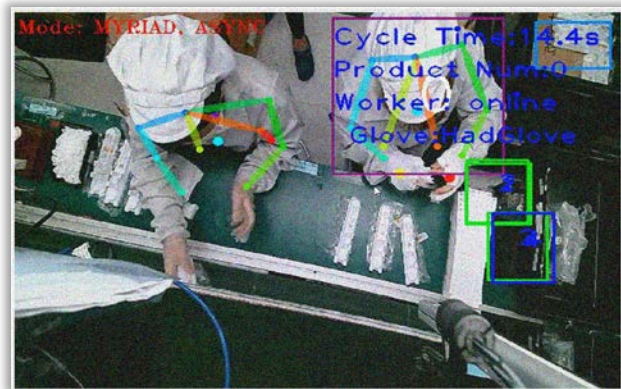
Figure 2. Live monitoring of the AMS
