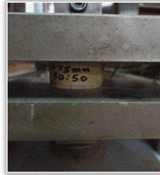
Figure 4: Compression strength samples under test
