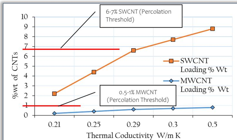
Figure 3. Thermal Conductivity vs. SWCNT & MWCNT Loading [24][26]
