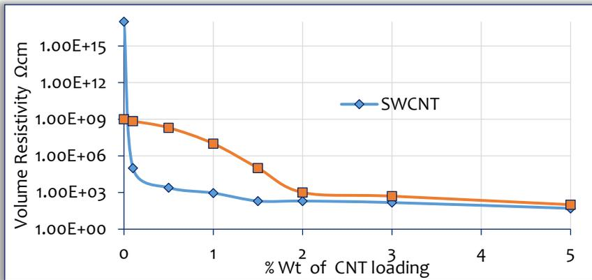
Figure 8. Volume Resistivity Vs amount of SWCNT & MWCNT [9]
