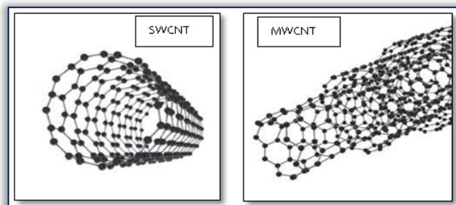
Figure 1. Single Walled Carbon Nanotube & Multi-walled Carbon Nanotubes [17]
