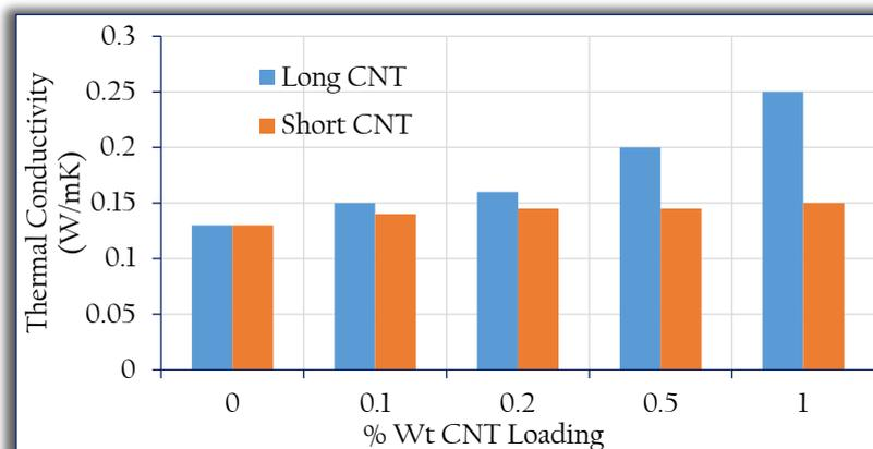
Figure 4. Thermal Conductivity vs. Long & Short CNT Loading [28]
