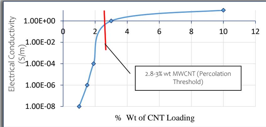
Figure 7. Electrical Conductivity Vs %wt MWCNT loading [27]
