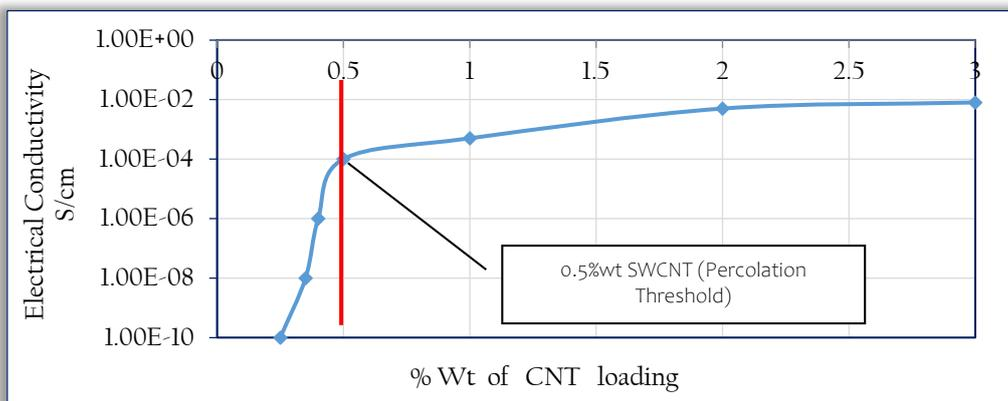
Figure 6. Electrical Conductivity Vs %wt SWCNT loading [29]
