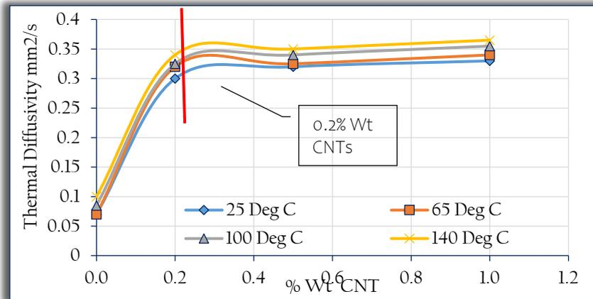
Figure 5. Thermal Diffusivity with temperature with different % of CNT amount [24]
